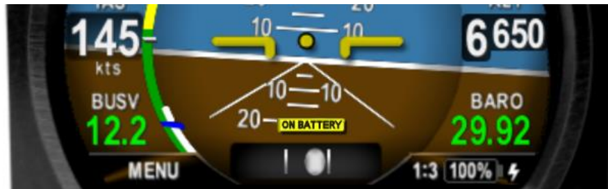
Figure 31 - On Battery Operation
