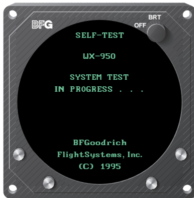
Figure 3-2. Self Test In Progress
