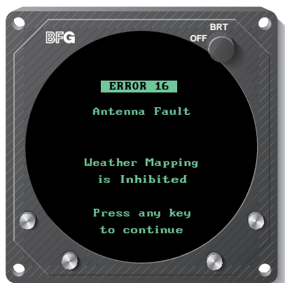
Figure 3-11. Error Message for a Recoverable Weather Fault
